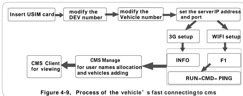
Figure 4-9, Process of the vehicle's fast connecting to cms
