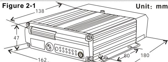
Function type MDVR dimension and installation hole site (double SD card machine), as shown in Figure 2-1
