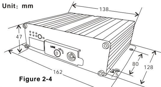
Simple type MDVR size and installation hole site (single/double SD card) as shown in Figure 2-4
