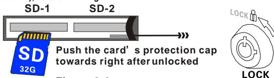
See Figure 2-2 : put the back of the SD card upside, insert it into the SD card slot, then pull on the card slot
