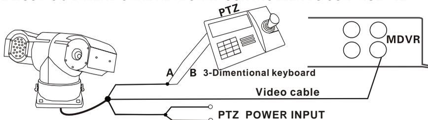
Figure 4-5: RS485 control line connect to the keyboard controller directly
