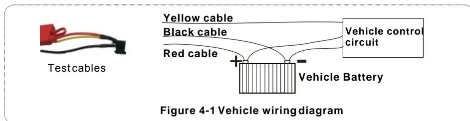
Figure 4-1 Vehicle wiring diagram
